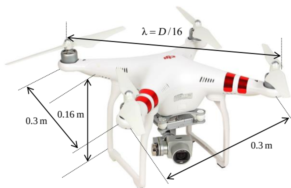
Fig. 2. General View of a Small-Sized Phantom 3 UAV
